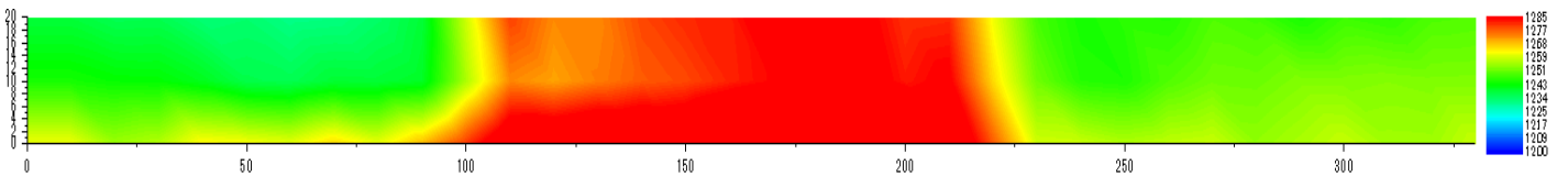
FIGURE 23: MAPPING OF THE INTENSITY OF INDUCED MAGNETIC FIELD USING THE PROBE N°3
