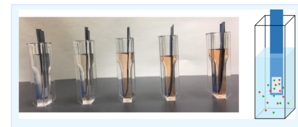
Reagent-deposited pieces of paper as reservoir for portable system
