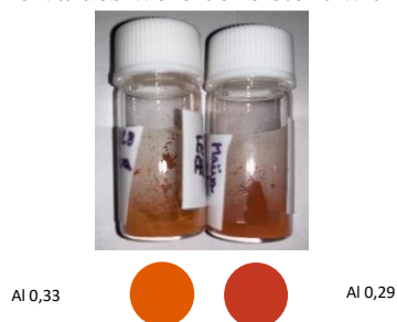
Picture 10: Color of 0,29 and 0,33 Al samples made with USP, at 800°C.
